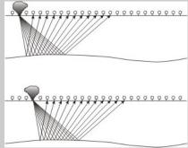
This laborious procedure is made efficient by placing a larger number of geophones on the ground connected through a rollalong switch to the seismograph. The switch electrically selects groups of geophones, eliminating the need to physically move them each time.
