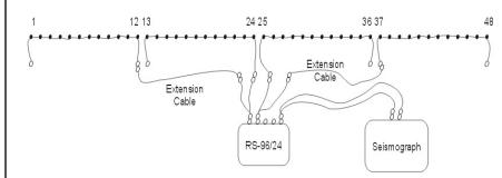
Shown here is the most popular configuration for surveys with a 24channel seismograph and an RS-96/24 rollalong switch. In this case, there are 48 geophones planted in the ground. The geophones are connected to four standard, 12-takeout refraction cables. Usually the user will have at least two already.
