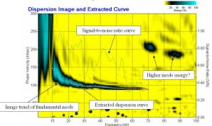
Inversion of Extracted Dispersion Curve for Vs Profile
