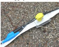
attach the anti-rotation wing supplied with the system to add stability.
