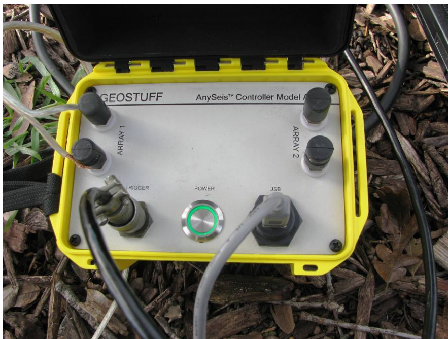
Controller module interfaces the seismic spread to the computer through the USB port. Also connects to the hammer switch. Small 12-volt battery powers string of geophone stations.
