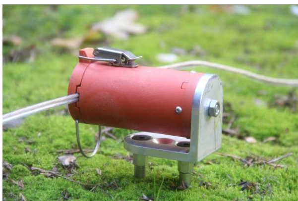
Conduct shear wave surveys with optional bracket. Standard 15-Hz sensor operates in either orientation.
