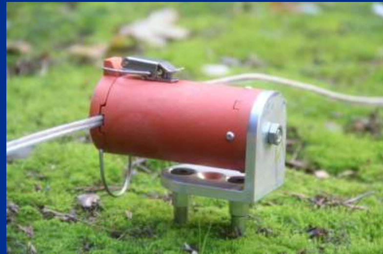
Optional right-angle bracket for shear waves (elevated to show dual spikes) Center hole attaches to land streamer
